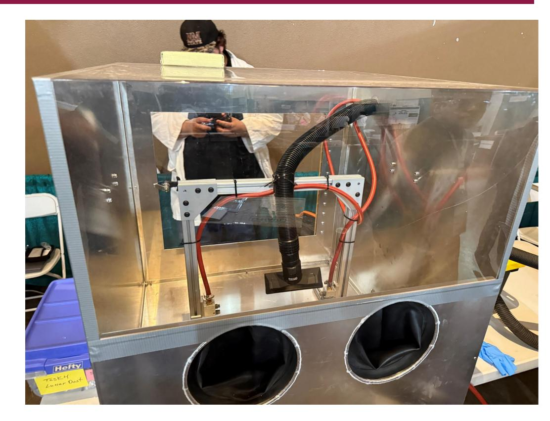
The final design includes a compact, modular decontamination chamber. It uses stationary air nozzles and a cyclone vacuum system. The key components are:
